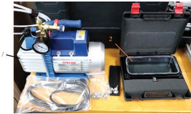
Figure 4. Appearance of vacuum detachable chamber (1) and compressor (2)
