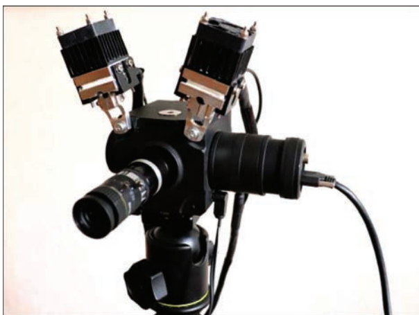
Figure 2. Appearance of shearography interferometer with laser modules
