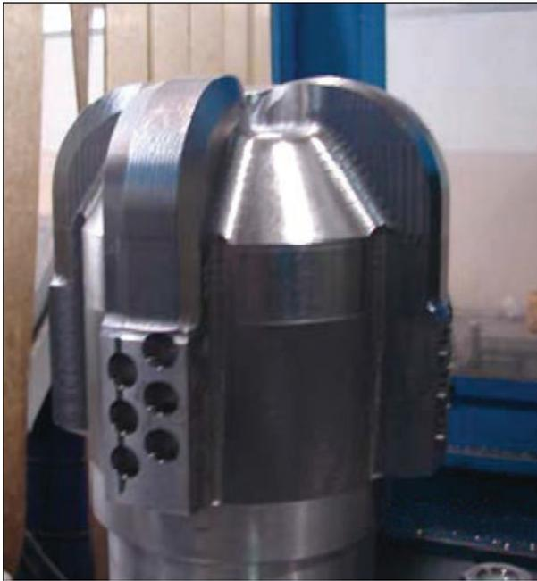
Figure 4. Frame of an integrally-milled bit
