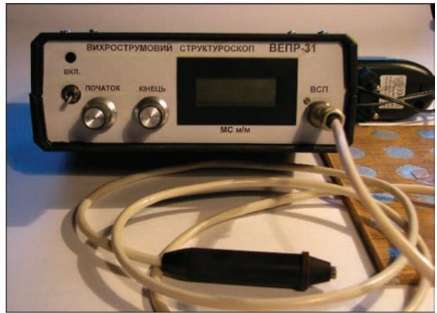
**Figure 4.** Eddy current structurescope of type VEPR-31
