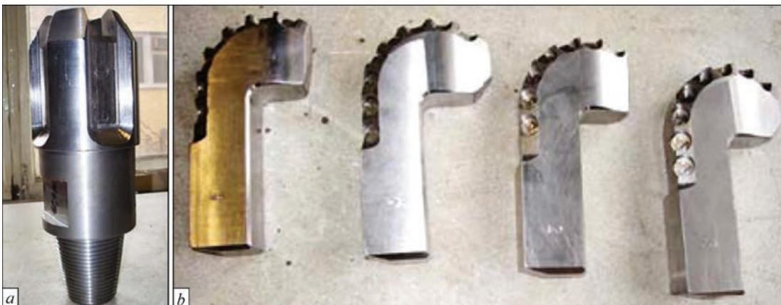
Figure 5. Combined bit: *a* — frame; *b* — blades
