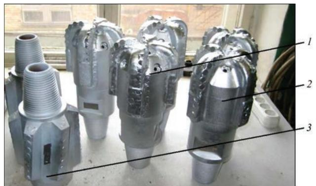
**Figure 8.** Drill bits with a protective coating: *1* — combined bit; *2* — integrally-milled bit; *3* — calibrator
