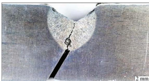
Figure 2. Cross-section of an underwater weld [11]
