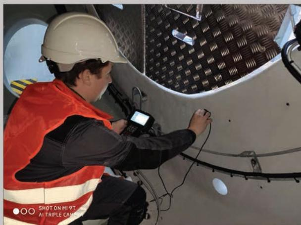
Ultrasonic testing of wind turbine hub
