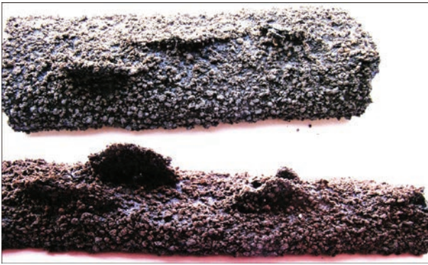
Figure 3. Unevenness of slag crust surface arising at excessive distance from CW to the last electrode
