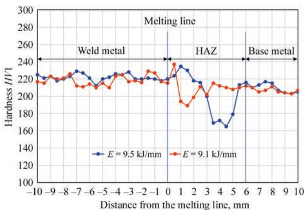
**Figure 6.** Hardness profile  $HV1$  in the weld seam during five-wire SAW welding for  $E = 9.5$  kJ/mm und  $E = 9.1$  kJ/mm, outer seam, tube wall thickness 39 mm
