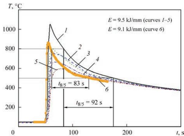
**Figure 5.** Welding temperature cycles for five-wire SAW welding for  $E = 9.5$  kJ/mm und  $E = 9.1$  kJ/mm, outer seam, tube wall thickness 39 mm
