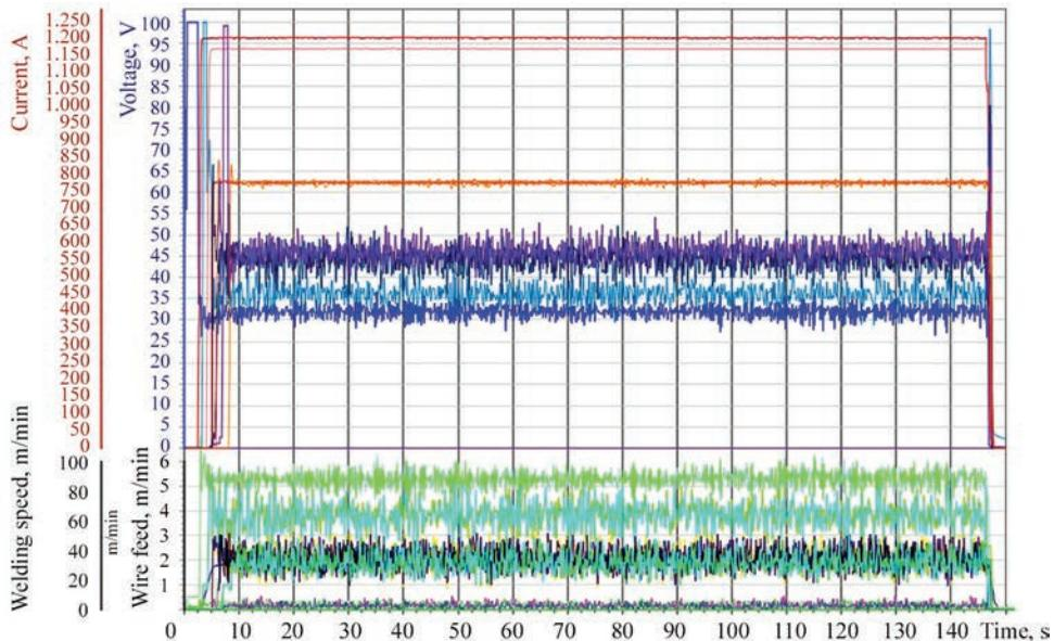
**Figure 4.** Recorded process data during five-wire SAW welding of a thick-walled pipe
