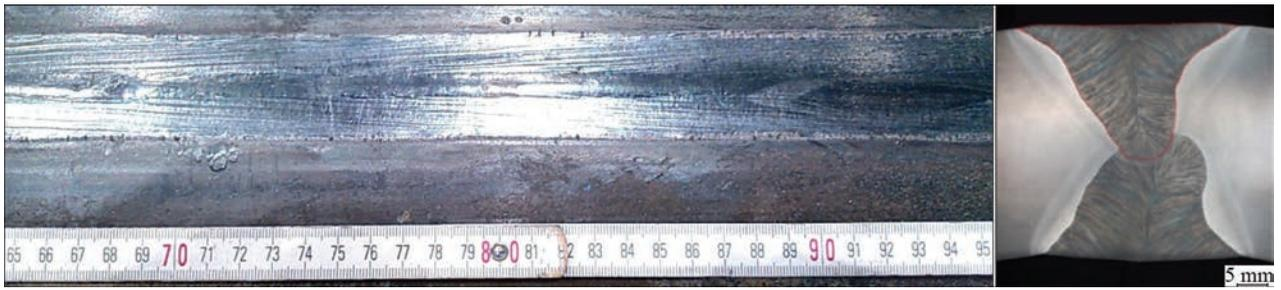
**Figure 3.** Outer appearance and cross-section of a SAW weld. Outer layer welded with the following wire configuration:  $d_1 = 3.2$  mm and  $d_{2,3,4,5} = 4$  mm; parameters:  $V = 1.2$  m/min,  $I_1 = 1200$  A,  $U_1 = 32$  V;  $I_2 = 1150$  A,  $U_2 = 36$  V;  $I_3 = 780$  A,  $U_3 = 42$  V;  $I_4 = 760$  A,  $U_4 = 44$  V;  $I_5 = 760$  A,  $U_5 = 44$  V
