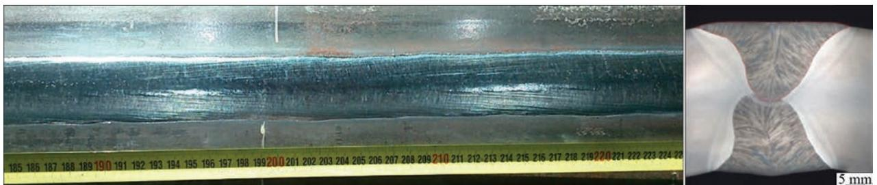
**Figure 2.** Outer appearance and cross-section of a SAW-weld. Outer layer welded with the following wire configuration:  $d_{1,2} = 4.8$  mm and  $d_{3,4,5} = 4$  mm; parameters:  $V = 1.1$  m/min,  $I_1 = 1480$  A,  $U_1 = 34$  V;  $I_2 = 1200$  A,  $U_2 = 38$  V;  $I_3 = 760$  A,  $U_3 = 38$  V;  $I_4 = 650$  A,  $U_4 = 38$  V;  $I_5 = 650$  A,  $U_5 = 38$  V
