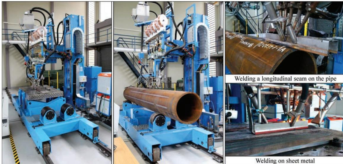
**Figure 1.** Five-wire SAW test stand for welding sheets and tubes at Fraunhofer IPK in Berlin
