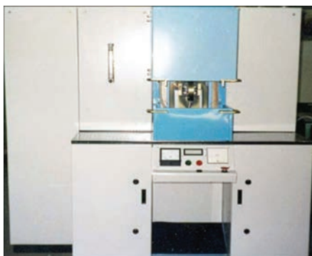
Figure 3. Installation H-126A for magnetic-pulse welding
