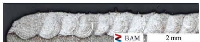
**Figure 3.** Cross section of buttering of edges
