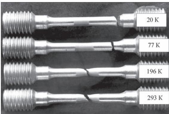
**Figure 5.** Nature of destruction of specimens cut from welded joints of stamped semi-finished product of the 1570 alloy at different test temperatures
