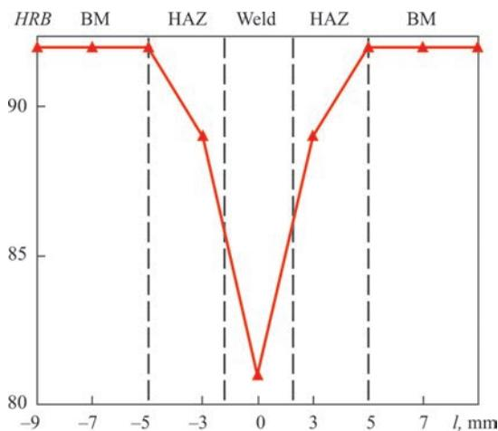
**Figure 2.** Distribution of hardness in the cross-section of joints of stamped semi-finished products of the 1570 alloy
