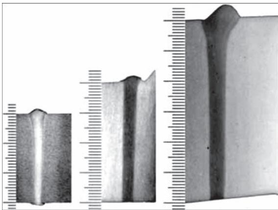
**Figure 1.** Macrosections of joints of semi-finished products of the 1570 alloy with a thickness of 30, 40 and 60 mm
