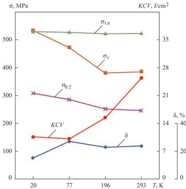
**Figure 4.** Dependence of mechanical properties of stamped semi-finished product of the 1570 alloy with a thickness of 60 mm on the test temperature
