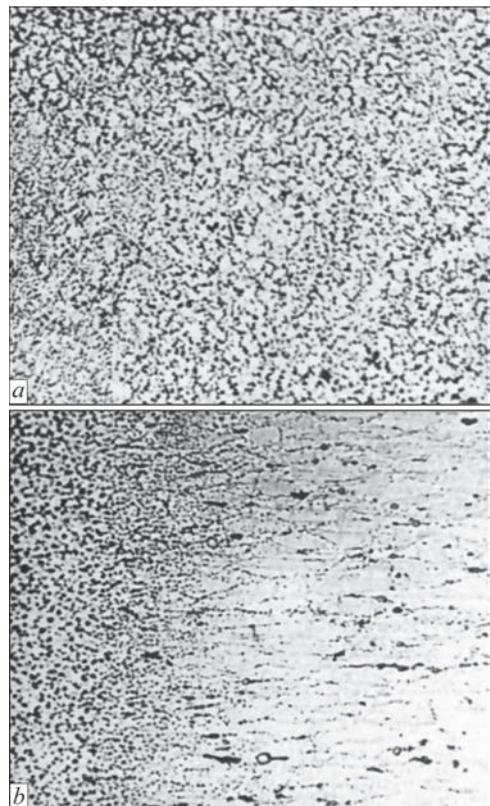
**Figure 3.** Microstructure ( $\times 200$ ) of weld metal of stamped semi-finished product of the 1570 alloy: *a* — central part of the weld; *b* — fusion line
