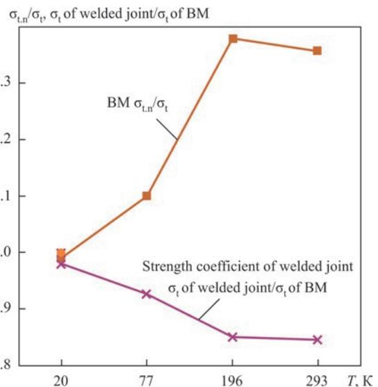
**Figure 7.** Effect of test temperature on strength coefficient of joints and sensitivity to stress concentrators of stamped semi-finished product of the 1570 alloy
