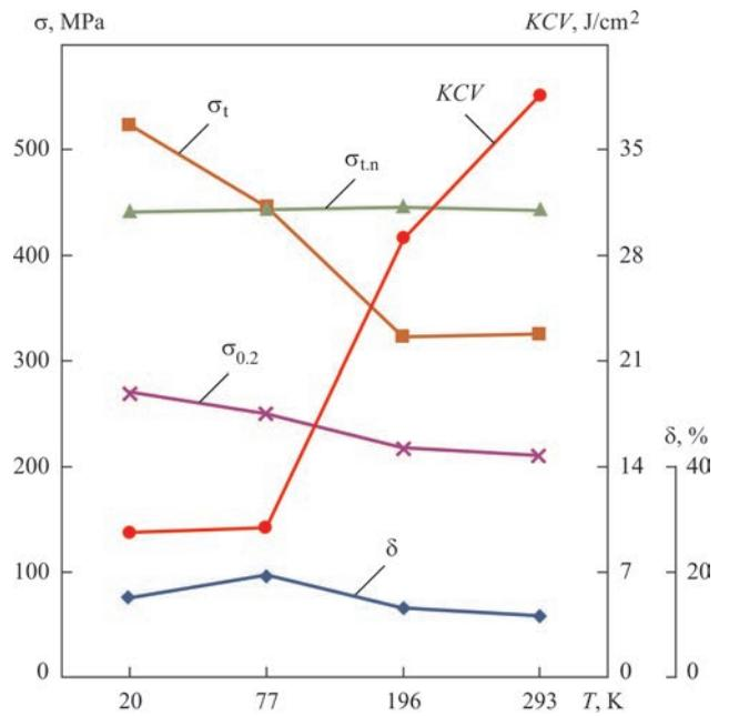
**Figure 6.** Dependence of mechanical properties of welded joints of the 1570 alloy, made by EBW method, on test temperature
