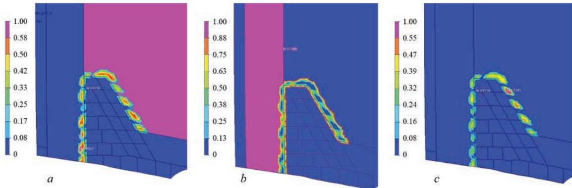
**Figure 5.** Results of modeling residual microstructural composition in the CWJ zone at  $T_{preheating} = 100 \text{ }^\circ\text{C}$ : *a* — bainite; *b* — ferrite-pearlite; *c* — martensite
