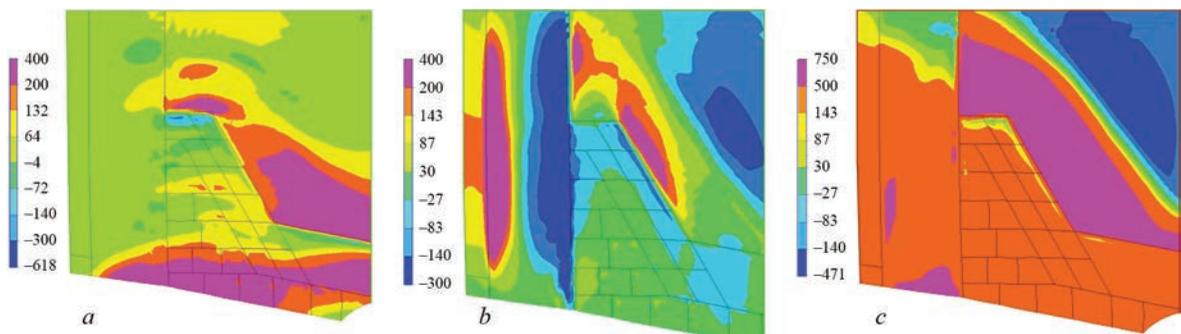
**Figure 7.** Residual stresses in CWJ after welding at  $T_{\text{heating}} = 100\text{ }^{\circ}\text{C}$ : *a* — radial; *b* — axial; *c* — circular
