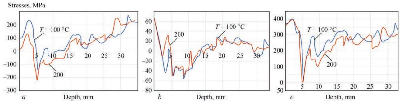
Figure 10. Effect of heating temperature during welding on distribution of residual stresses over the depth of the weld (cross-section *b–b* Figure 9): *a* — radial; *b* — axial; *c* — circular
