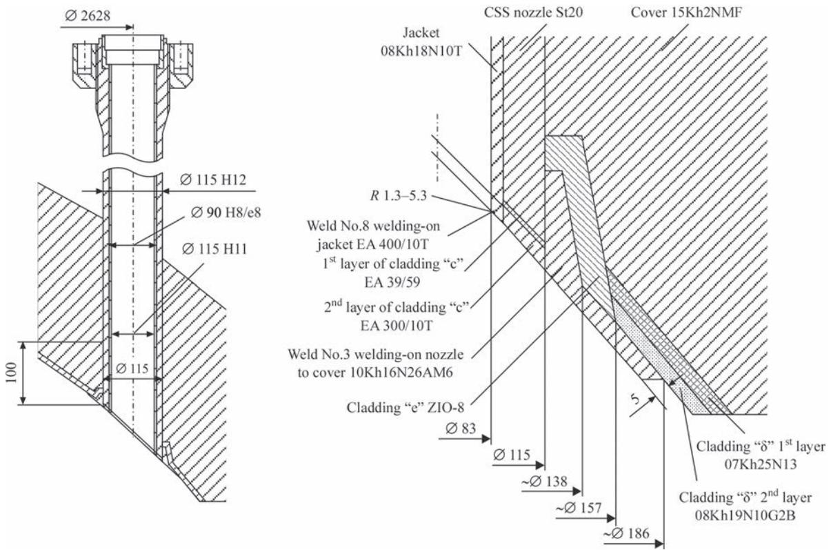
**Figure 1.** Reactor cover element with connected CSS nozzle and scheme of CWJ
