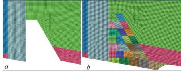
**Figure 3.** Finite element mesh in the CWJ zone: *a* — before welding; *b* — after welding
