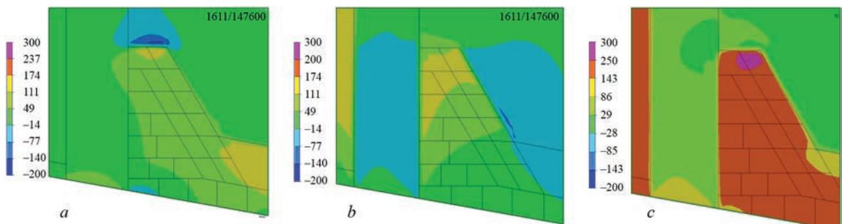
**Figure 8.** Residual stresses in CWJ after welding ( $T_{\text{heating}} = 100\text{ }^{\circ}\text{C}$ ) and heat treatment ( $T = 650\text{ }^{\circ}\text{C}$ ,  $t_{\text{holding}} = 15\text{ h}$ ): *a* — radial; *b* — axial; *c* — circular
