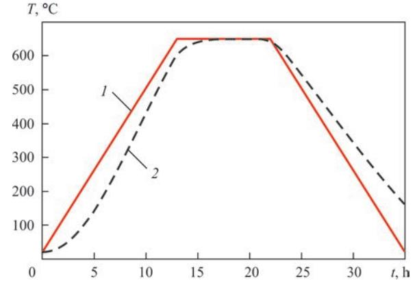
**Figure 4.** Diagram of changing temperature of CWJ material in the process of heat treatment using a high tempering mode at  $T = 650 \text{ }^\circ\text{C}$ : 1 — heat treatment mode; 2 — calculated temperature where the rate of creep deformations was determined by the Bailey–Norton’s law [13]:
