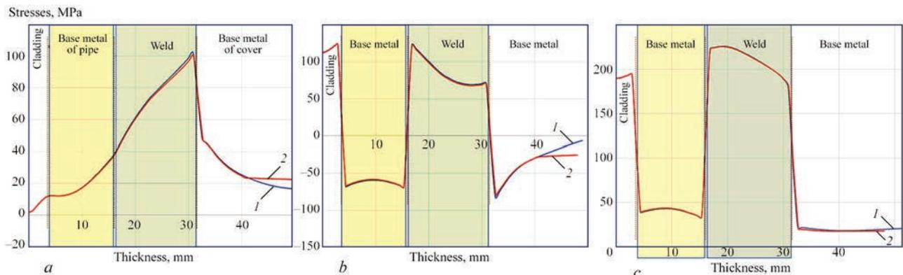
Figure 12. Effect of holding time during heat treatment ( $T = 650\text{ }^{\circ}\text{C}$ ) on distribution of residual stresses across the width of the weld (cross-section *a–a* Figure 9): *a* — radial; *b* — axial; *c* — circular; 1 — 15 h; 2 — 9
