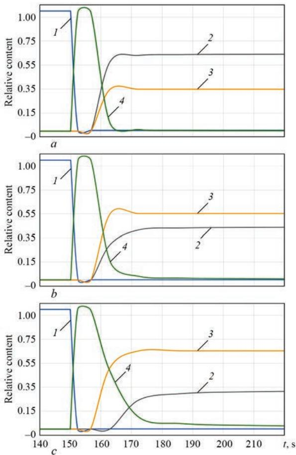
**Figure 6.** Kinetics of microstructural phase transformations at the characteristic point of HAZ of the base material of the cover (15Kh2NMFA steel) for different preheating temperatures: *a* — without preheating; *b* —  $T_{\text{preheating}} = 100\text{ }^{\circ}\text{C}$ ; *c* —  $T_{\text{preheating}} = 200\text{ }^{\circ}\text{C}$ ; 1 — ferrite; 2 — martensite; 3 — bainite; 4 — austenite
