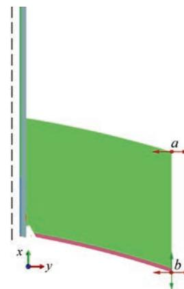
**Figure 2.** Boundary conditions and scheme of 2D model of CWJ:  $a$  — restricts movement in the horizontal plane;  $b$  — restricts movement in the horizontal and vertical planes
