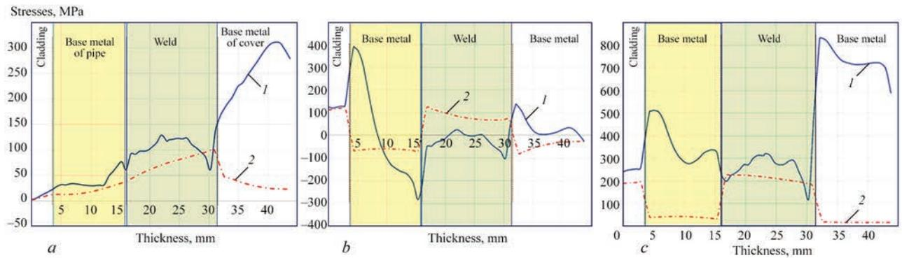
Figure 11. Effect of heat treatment ( $T = 650\text{ }^{\circ}\text{C}$ ) on distribution of residual stresses across the width of the weld (cross-section *a–a* Figure 9): *a* — radial; *b* — axial; *c* — circular; 1 — before heat treatment; 2 — after heat treatment
