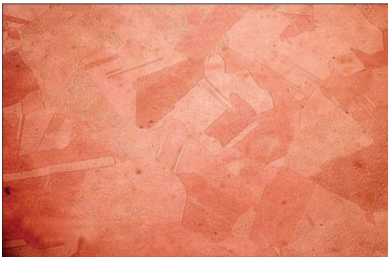
Figure 2. Microstructure ( \times 200 ) of copper used as a base metal
