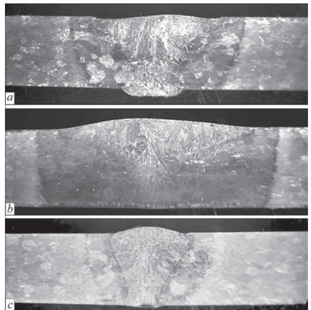
**Figure 1.** Transverse macrosections of welded joints of 8 mm thickness of a high-temperature pseudo- $\alpha$  titanium Ti-5.6Al-2.2Sn-3.5Zr-0.4Mo-1.0V-0.6Si alloy: *a* — AAW with the preheating to 200 °C (mode No. 1); *b* — AAW with the preheating to 400 °C (mode No. 2); *c* — AAW over the flux with the preheating to 200 °C (mode No. 3)
