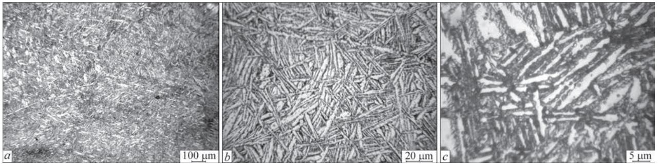
**Figure 2.** Microstructure of base metal of a high-temperature pseudo- $\alpha$  titanium Ti-5.6Al-2.2Sn-3.5Zr-0.4Mo-1.0V-0.6Si alloy (description *a-c* see in the text)
