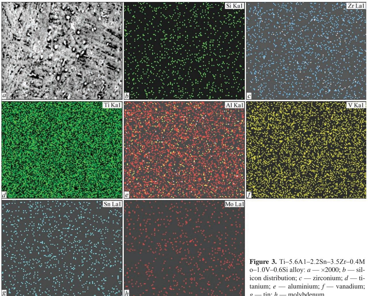
**Figure 3.** Ti-5.6Al-2.2Sn-3.5Zr-0.4Mo-1.0V-0.6Si alloy: *a* —  $\times 2000$ ; *b* — silicon distribution; *c* — zirconium; *d* — titanium; *e* — aluminium; *f* — vanadium; *g* — tin; *h* — molybdenum
