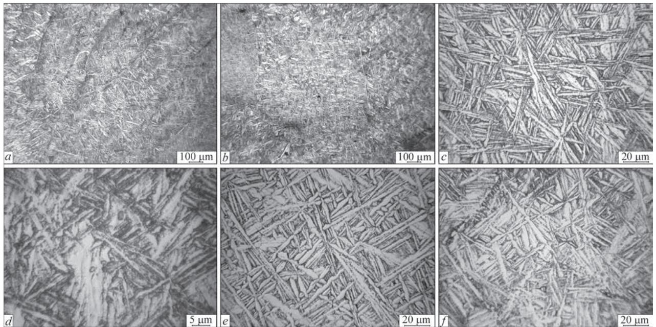
**Figure 6.** Microstructure of metal of HAZ joints of a high-temperature pseudo- $\alpha$  titanium Ti-5.6Al-2.2Sn-3.5Zr-0.4Mo-1.0V-0.6Si alloy, produced by AAW in the state after welding: *a-c* — mode No. 3 (400 °C); *d, e* — No. 2 (200 °C); *f* — No. 4 over the flux (200 °C)
