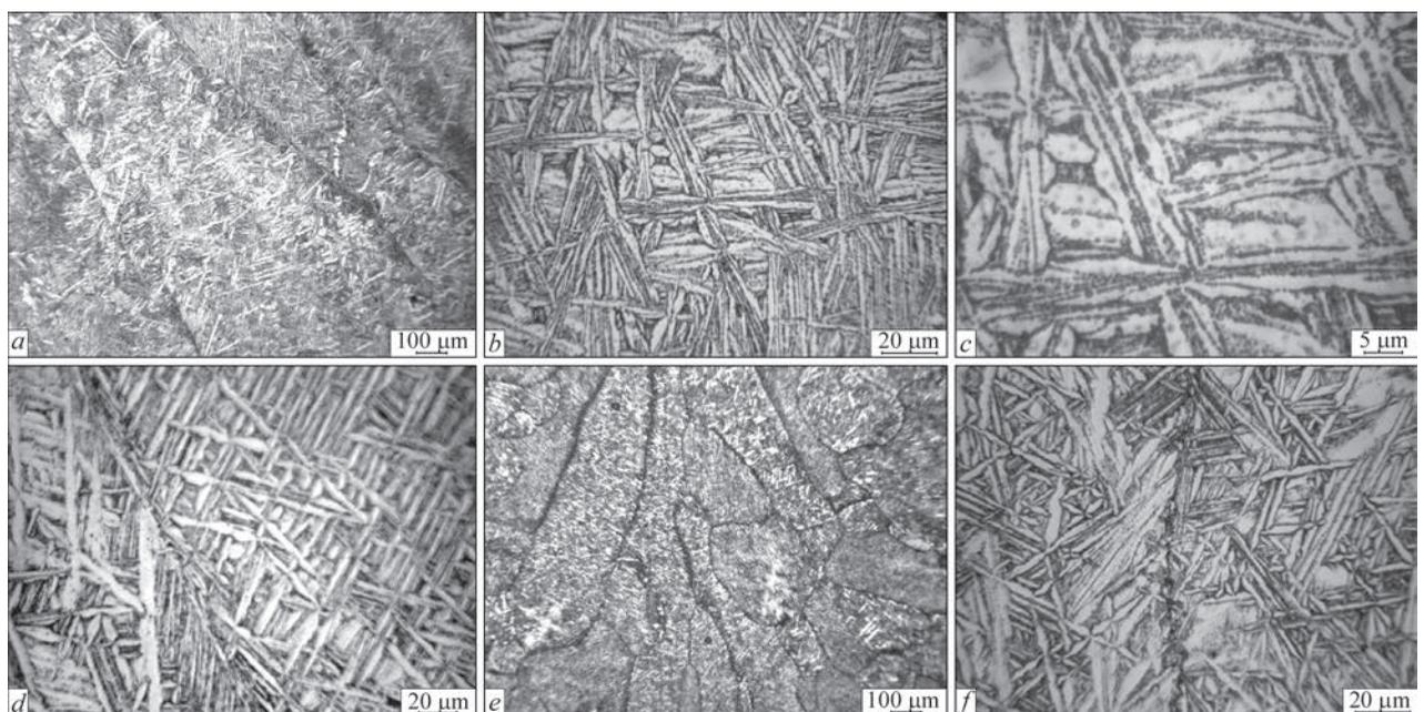
**Figure 5.** Microstructure of weld metal of joints of a high-temperature pseudo- $\alpha$  titanium Ti-5.6Al-2.2Sn-3.5Zr-0.4Mo-1.0V-0.6Si alloy, produced by AAW in the state after welding: *a-c* — mode No. 2 (400 °C); *d* — No. 1 (200 °C); *e, f* — No. 3 over the flux (200 °C)
