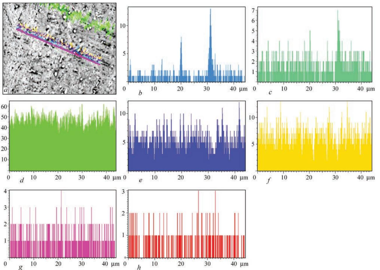
**Figure 4.** Ti-5.6Al-2.2Sn-3.5Zr-0.4Mo-1.0V-0.6Si alloy: *a* —  $\times 2000$ ; *b* — spectrum of silicon; *c* — zirconium; *d* — titanium; *e* — aluminium; *f* — vanadium; *g* — tin; *h* — molybdenum
