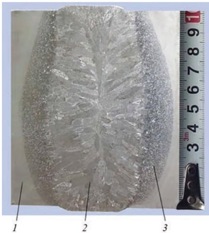
**Figure 3.** Macrostructure of welded joint (cross-section): 1 — BM; 2 — weld; 3 — HAZ
