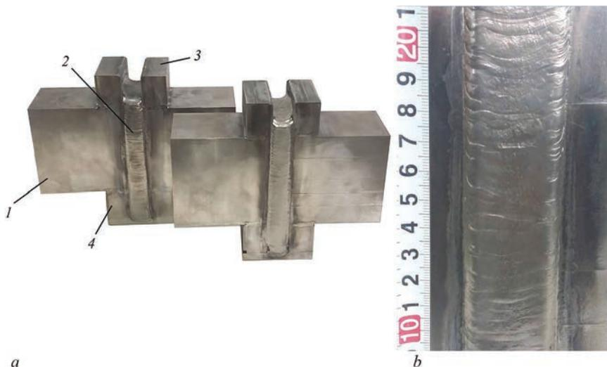
**Figure 2.** Appearance of welded joints (a) and weld surface (b): 1 — base metal; 2 — weld; 3, 4 — technological straps
