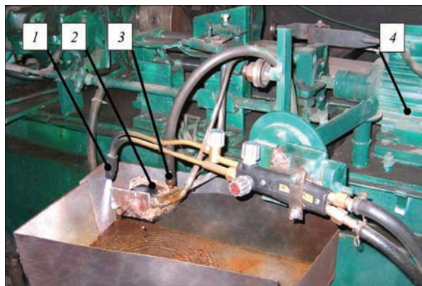
Figure 2. Appearance of the installation unit for studying heat resistance of the deposited specimens: 1 — gas torch for heating of the specimen; 2 — tested specimen; 3 — hose for supplying water that cools the specimen; 4 — drive for movement of the specimen
