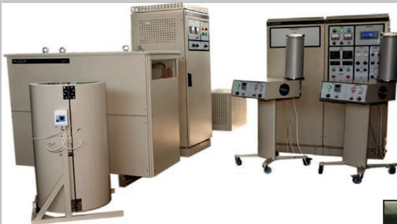
The equipment is designed for applying wear-resistant, corrosion-resistant, heat-shielding and special coatings by spraying powders from metals, alloys, carbides, borides, oxides and metal-ceramic materials. The thickness of applied coatings is from 20–50  $\mu\text{m}$  to 1–2 mm and more.
