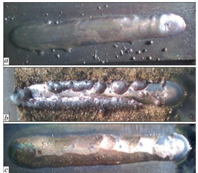
**Figure 4.** Appearance of deposited beads: *a* — surfacing in argon; *b* — argon + 4.0 mm of flux AN-60SM; *c* — argon + 6.0 mm of flux AN-60SM
