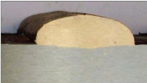
**Figure 7.** Transverse macrosection of deposited bead of bronze at optimal modes ( $\times 2$ )
