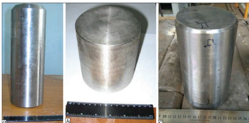
Figure 3. Appearance of ingots of Ti-Al-Zr-Si-Mo-Nb-Sn system titanium alloys of 110 mm diameter after side surface machining: a — 812-208 melt; b — 814-208 melt; c — 815-208 melt
