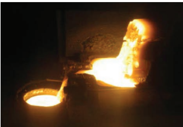
Figure 1. Process of melting of ingot of Ti–Al–Zr–Si–Mo–Nb–Sn system titanium alloy of 110 mm diameter in electron beam unit
