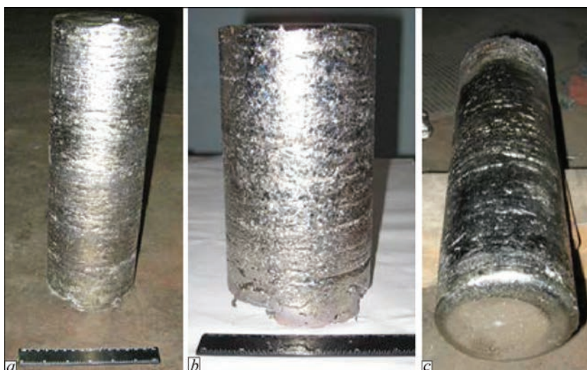
Figure 2. Ingots of Ti-Al-Zr-Si-Mo-Nb-Sn system titanium alloys of 110 mm diameter after EBM: a — 812-208 melt; b — 814-208 melt; c — 815-208 melt
