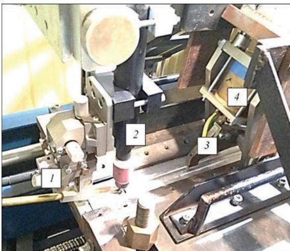
**Figure 2.** Hardware complex for automatic TIG welding which is compatible with weld EDT: 1 — system for filler wire feeding; 2 — welding torch; 3 — electrode device; 4 — linear displacement solenoid of EDT electrode
