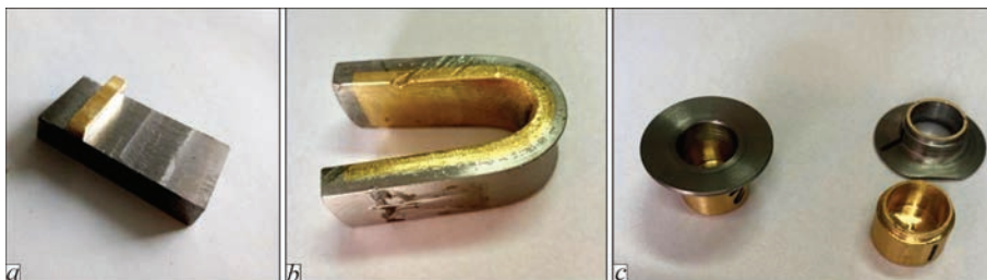
Figure 8. Samples for mechanical testing of brass–steel joints: a — shear testing of cladding layer; b — two-layer joint after static bend testing with cladding layer inside; c — before and after cladding layer tearing tests
