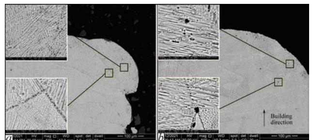
**Figure 2.** Porosity at negative (*a*) and positive (*b*) defocusing amount [27]
