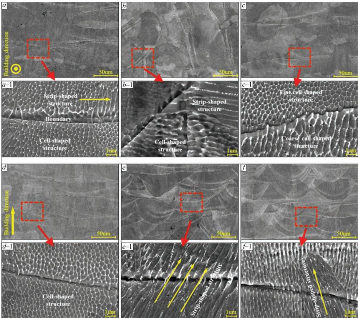
**Figure 4.** SEM micrograph of specimens: *a, d* — XY and XZ planes with strategic rotation angle of  $0^\circ$ ; *b, e* — XY and XZ planes with strategic rotation angle of  $67.5^\circ$ ; *c, f* — XY and XZ planes with strategic rotation angle of  $90^\circ$  [34]
