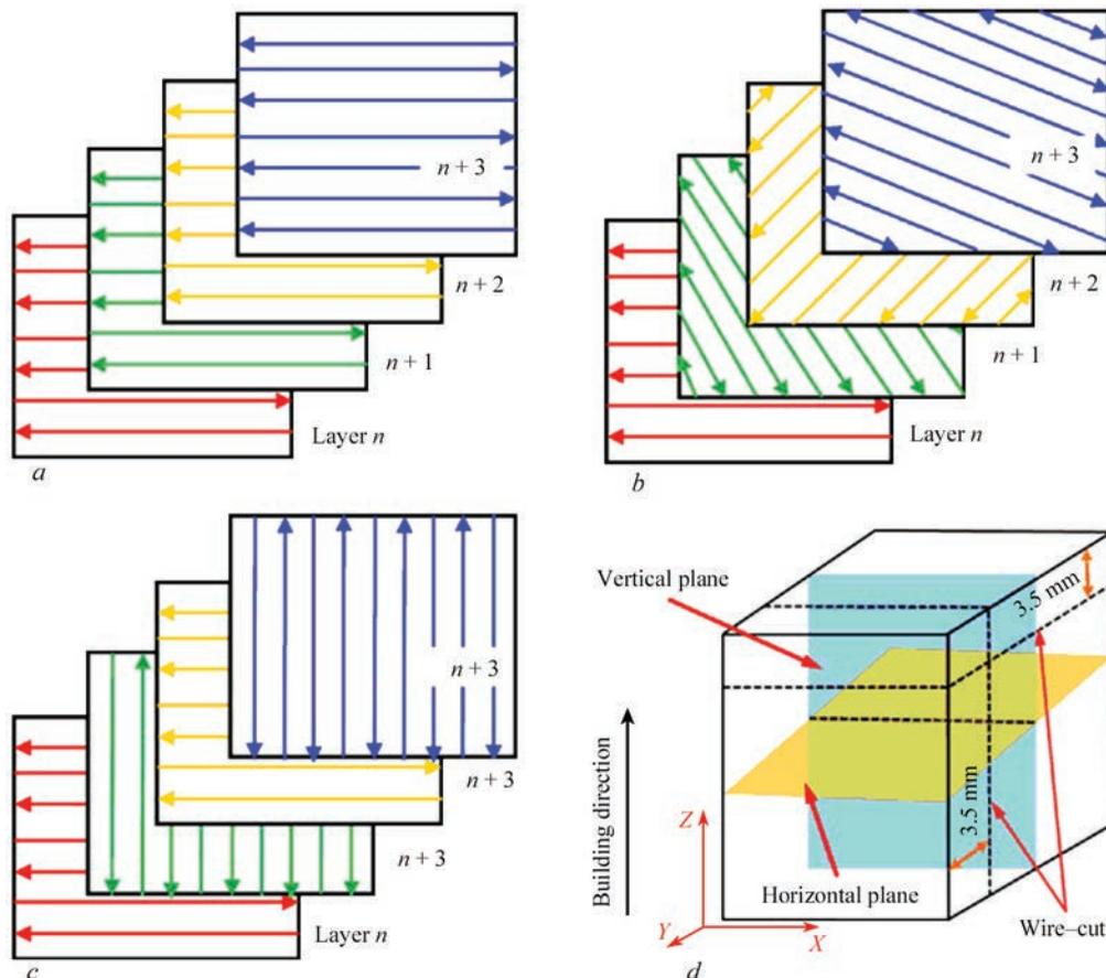
**Figure 3.** Scanning strategies used in [33]: *a* — without rotation; *b* — with rotation by  $67.5^\circ$ ; *c* — with rotation by  $90^\circ$ ; *d* — indication of vertical and horizontal planes
