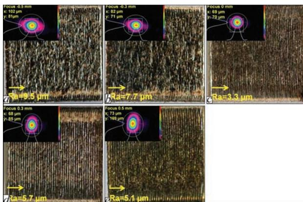
**Figure 1.** Macroscopic top view of SLM specimens produced with different defocusing amount, mm: *a* —  $-0.5$ ; *b* —  $-0.3$ ; *c* —  $0$ ; *d* —  $0.3$ ; *e* —  $0.5$  [25]
