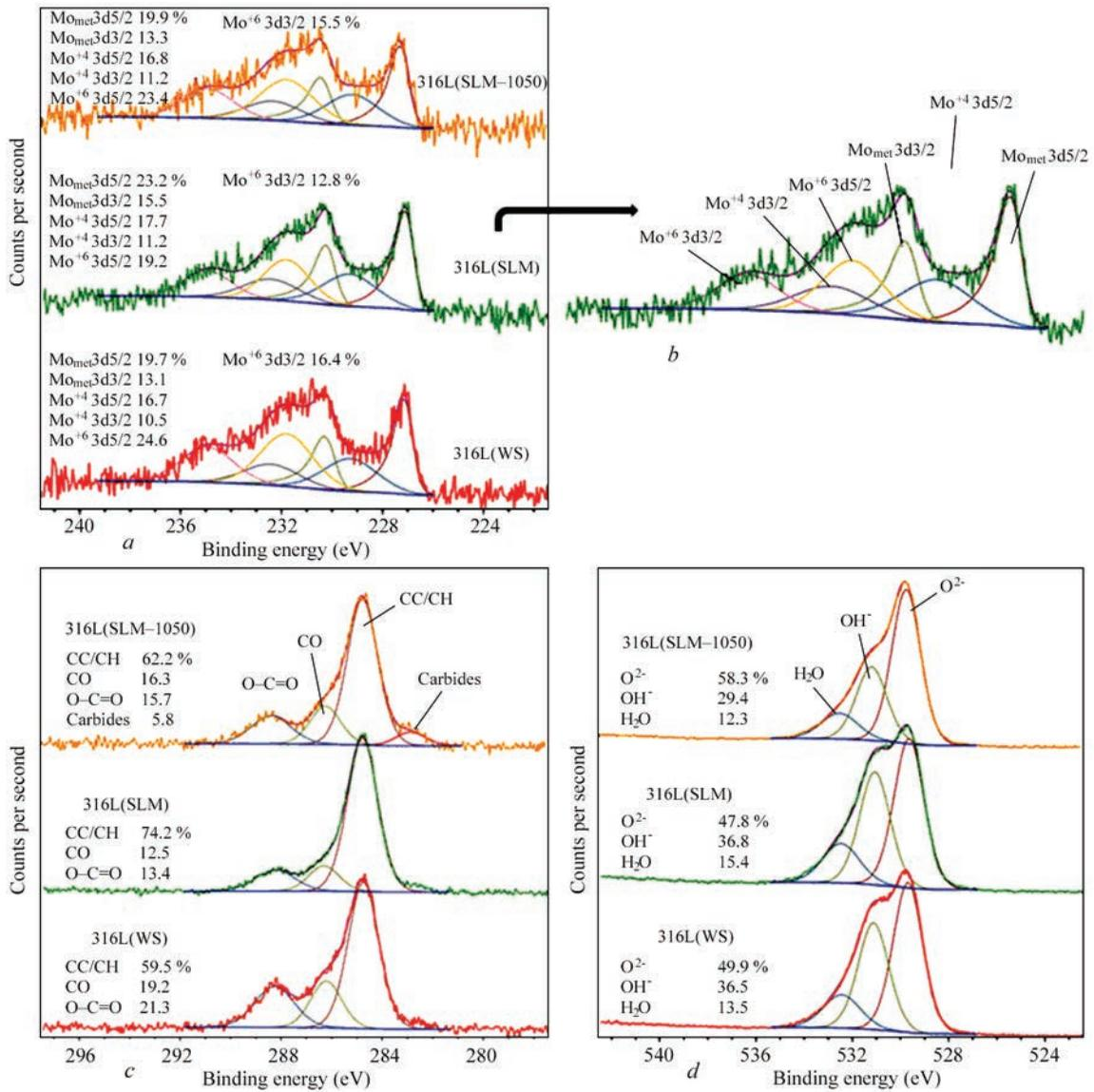
**Figure 6.** XPS-spectroscopy results of varieties of 316L steel after surface treatment: *a, b* — molybdenum levels; *c* — carbide levels; *d* — oxide levels [46]
