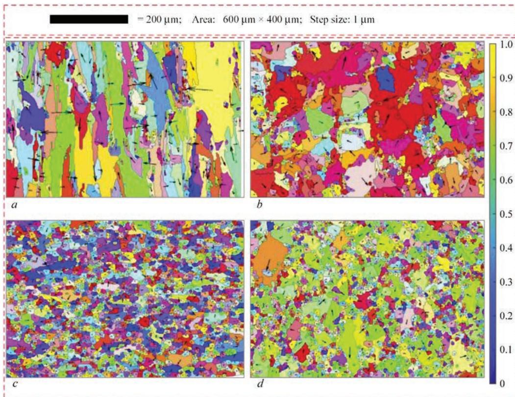
**Figure 5.** Grain microstructure in deformed (*b, d*) and undeformed (*a, c*) specimens of Inconel 718 alloy, produced by forging (*c, d*) and selective laser melting (*a, b*) technologies [42]
