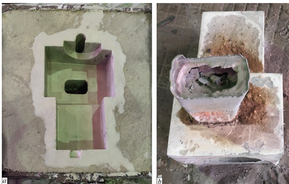
Figure 5. Production of massive shaped fluorophlogopite castings: a — sand-clay mould; b — fluorophlogopite casting of “tap-hole stone” for chlorinator with a total weight of 150 kg
