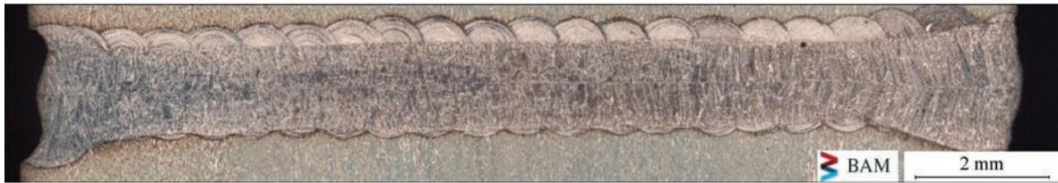
**Figure 4.** Microsection of weld seam with LMD-tacking
