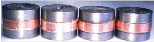
Figure 6. Specimens joined by MPW
