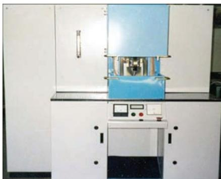
**Figure 3.** Installation H-126A for magnetic-pulse welding
