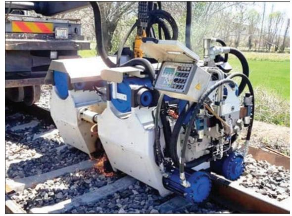
**Figure 6.** Welding head AMS100
