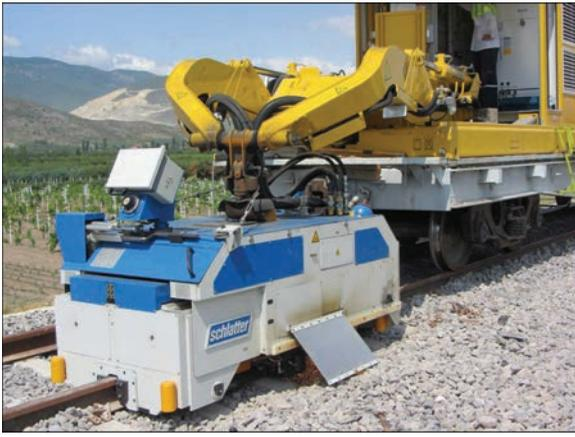
**Figure 5.** Container system Multiflex for welding rails with welding head AMS60
