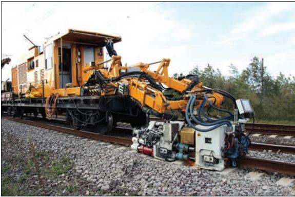
Figure 8. Welding machine of container type ART1500RC
