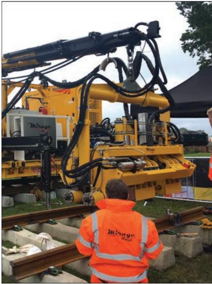
**Figure 10.** Induction welding robot of Mirage Rail Company of rails is carried out throughout the whole perimeter by the currents of magnetic induction with the help of inductors. The power consumption is 150 kVA.
