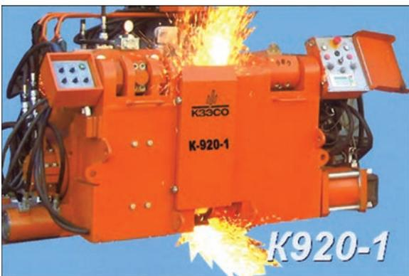
**Figure 2.** Rail welding head K920-1
