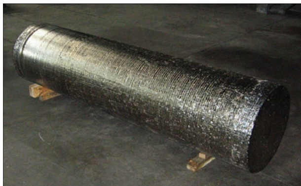
Figure 1. Ingot of VT9 alloy produced by EBM process
