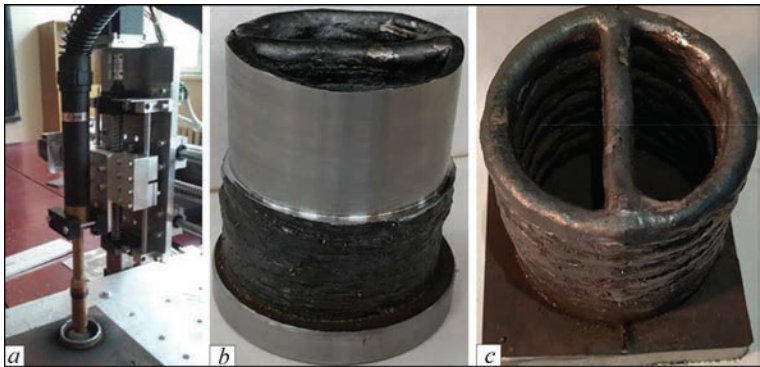
Figure 2. Head (a) with a consumable electrode for additive growing of parts with inner stiffeners (b, c)
