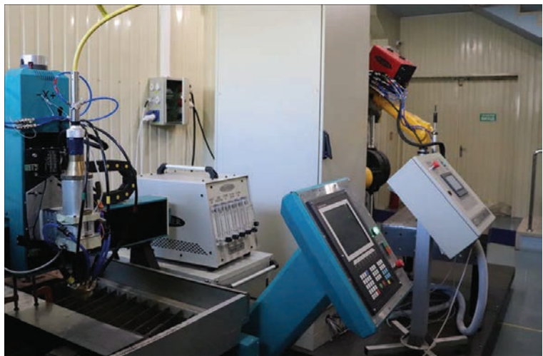
Figure 8. Universal technological complex for laser and hybrid laser-plasma cutting
