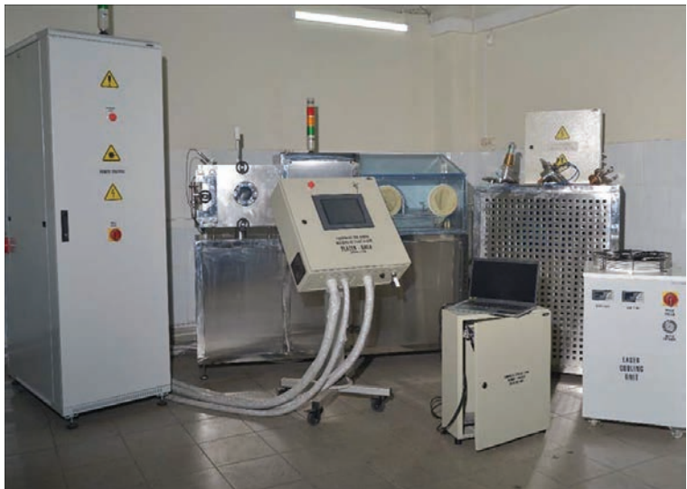
Figure 9. Complex for laser, microplasma and laser-microplasma welding in a controlled atmosphere and in a dynamic vacuum
