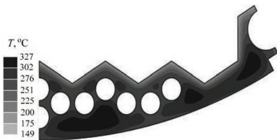
Figure 3. Temperature field at moment of time t = 100 s since ES start
