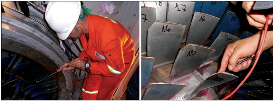
Figure 12. Maintenance testing of gas turbine blades using ECP of MDF 0501 type
