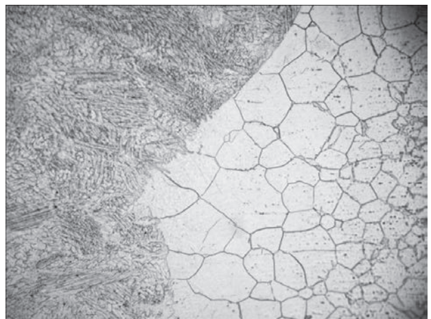
Figure 9. Microstructure ( \times 200 ) of HAZ metal and fusion line with the flange of welded T-joint after repair welding
