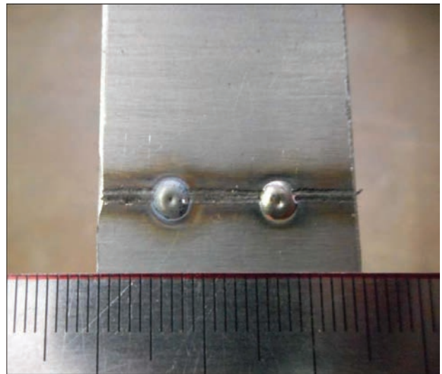
Figure 11. Photo of specimen for tests on static tension with repaired two spot defects
