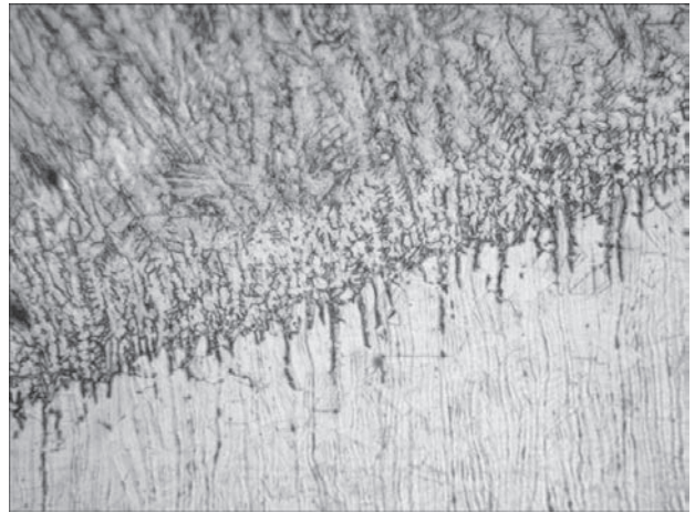
Figure 8. Microstructure ( \times 500 ) of initial weld and HAZ metal in the stiffener of welded T-joint after repair welding
