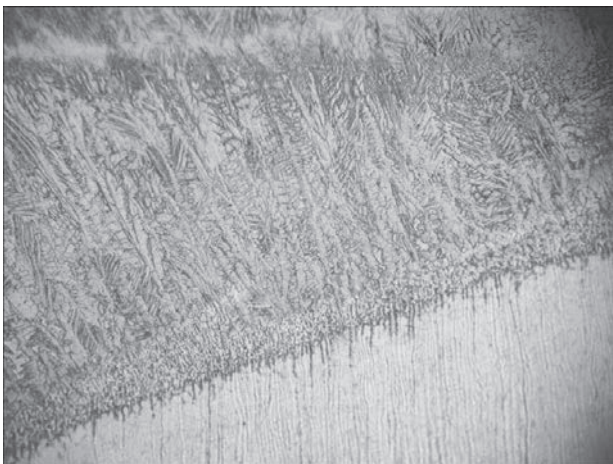
Figure 6. Microstructure ( \times 200 ) of initial weld and HAZ metal in the stiffener of welded T-joint after repair welding
