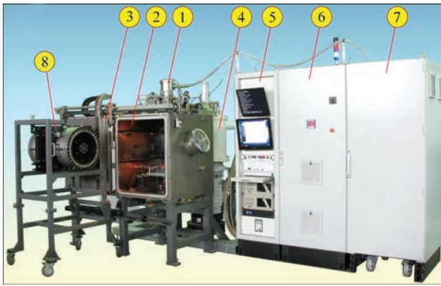
Figure 4. Installation for EBP of hard alloy billets, where: 1 — electron beam gun; 2 — vacuum chamber; 3 — sliding doors; 4 — vacuum system; 5 — control cabinet; 6 — power cabinet; 7 — welding high-voltage power source cabinet; 8 — loading device for two feed drums of parts
