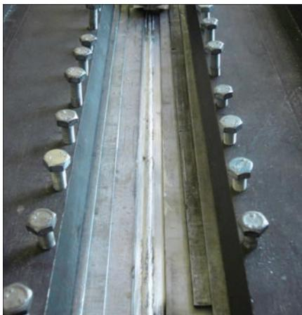
**Figure 3.** Appearance of welded joint of AMg5M alloy in the assembly and welding device immediately after plasma-arc welding at a variable polarity asymmetrical current at a speed of 200 cm/min
