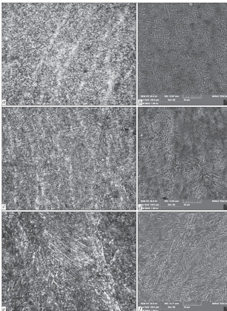
**Figure 5.** Structure of the upper weld layer in welding using stationary arc (*a, b*), in PAW (*c, d*) and pulsating arc (*e, f*): *a, c, e* — optic microscopy at  $\times 500$  (2 times decreased); *b, d, f* — CEM
