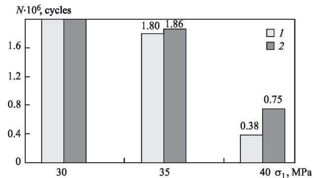
**Figure 7.** Resistance of T-welded joints of 13KhGMRB steel to fatigue cracks formation at cyclic bending load: 1 — stationary process; 2 — PAW
