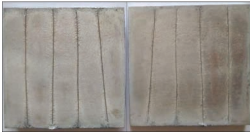
Figure 5. Surfaces of AMg6 alloy plates after thermal cycle of heating under the conditions of their compression with 100 kPa force
