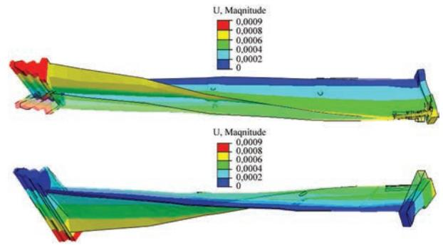
Figure 7. Blade residual deformations (torsional), up to 0.9 mm value of maximal displacements
