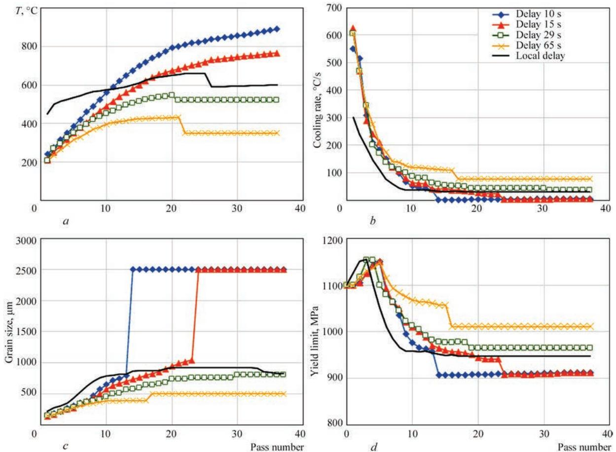
**Figure 4.** Dependence of temperature in a point before the next layer deposition (*a*), cooling rate (*b*), grain size (*c*) and material yield limit (*d*) on pass number for different interpass delay times [6]
