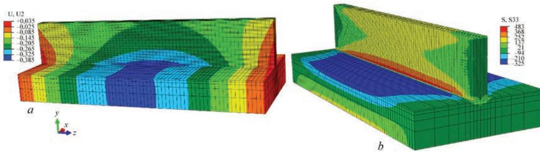
**Figure 3.** Results of calculation of residual stress-strain state in a tee sample [5]: *a* — longitudinal deflection; *b* — longitudinal stresses
