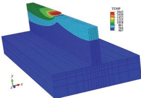
**Figure 2.** Results of calculation of temperature distribution in a tee sample during layer-by-layer formation of the part [5]
