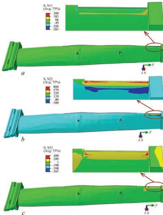
Figure 6. Residual stress distribution: *a* —  $\sigma_{xx}$  component by deposit height ( $\sigma_{xx} = 150\text{--}300$  MPa); *b* —  $\sigma_{yy}$  longitudinal component ( $\sigma_{yy} = -300\text{--}800$  MPa); *c* —  $\sigma_{zz}$  transverse component by blade thickness ( $\sigma_{zz} = -200\text{--}400$  MPa)
