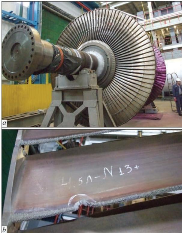
**Figure 1.** Erosion wear of a blade of the last stage of K-1000-60/3000 steam turbine LPC: *a* — general view of 5<sup>th</sup> stage; *b* — defect of blade edge erosion wear
