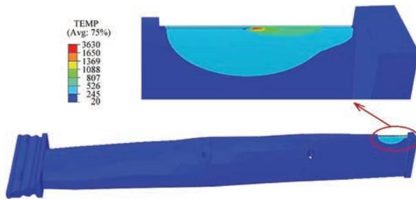
Figure 5. Temperature distribution during electron beam surfacing
