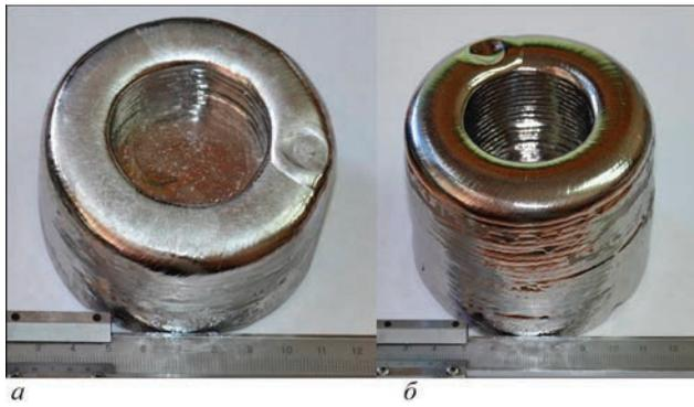
**Figure 7.** Tungsten single-crystal: *a* — after the first stage of deposition of 6 layers and surface etching; *b* — after the second stage of growing, the height of the wall is 35–37 mm
