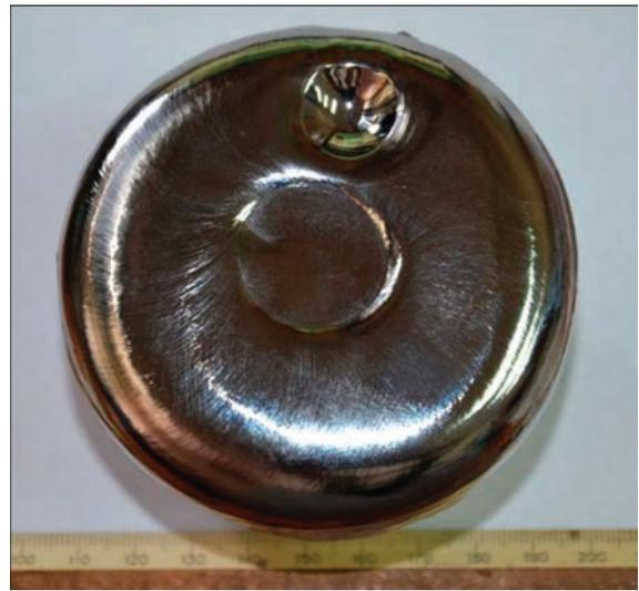
**Figure 5.** Outer surface of the embryonic crystal before the experiments on growing the walls of the hollow single-crystalline cylinder
