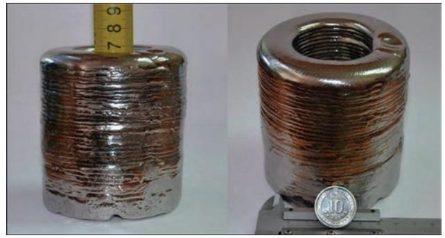
**Figure 8.** Appearance of tungsten single-crystal in the form of a hollow body of revolution of 85 mm diameter
