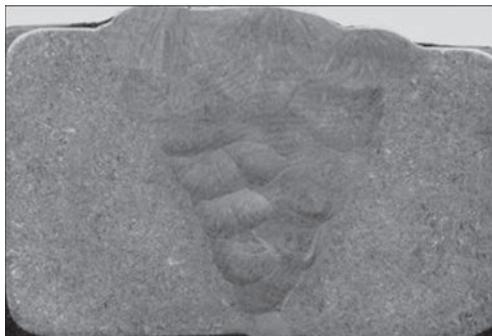
**Figure 4.** Macrosection of CA-6NM steel welded joint
