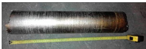
**Figure 8.** Ti-6Al-7Nb titanium alloy ingot of 110 mm diameter
