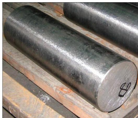
**Figure 9.** Machined ingot of Ti-6Al-7Nb titanium alloy
