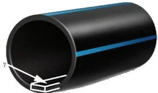
**Figure 3.** Direction of cutting out sections  $\gamma$  from the walls of polyethylene pipes for structural and thermophysical studies
