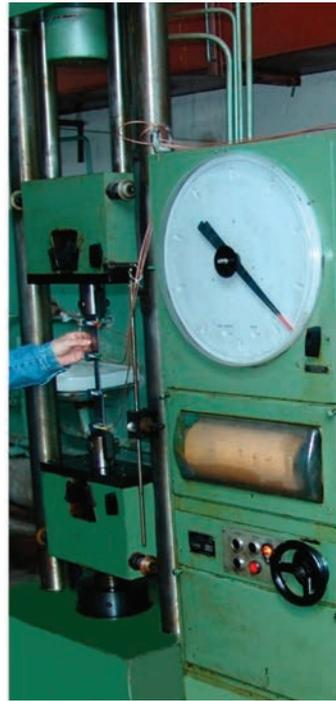
**Figure 1.** Sample and schematic of its mounting in R-20 machine
