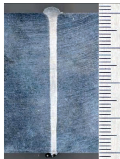
Figure 1. Transverse section of a joint of 2219 alloy plates 40mm thick
