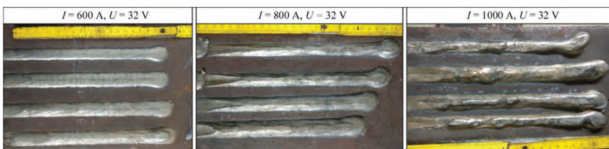
Figure 2. Outer appearance of bead on plates SAW welds produced with different parameters
