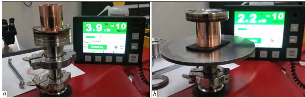
Figure 12. Measurement of the helium leakage of the conflate joint (a) and the contact surface between the deposited material (copper) and the substrate (stainless steel conflate) (b)
