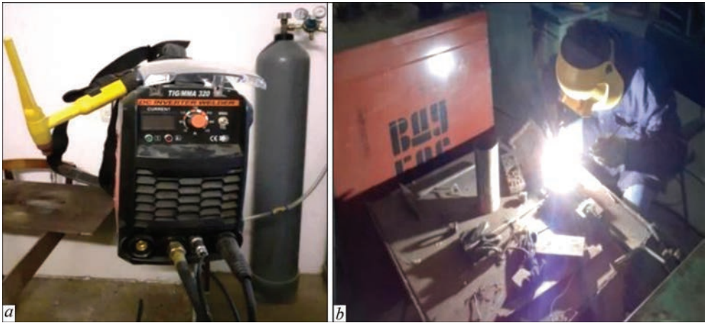
Figure 6. Inverter welding machine TIG/MMA-320 (a) and argon-arc welding process on universal welding rectifier VDU-506 (b)
