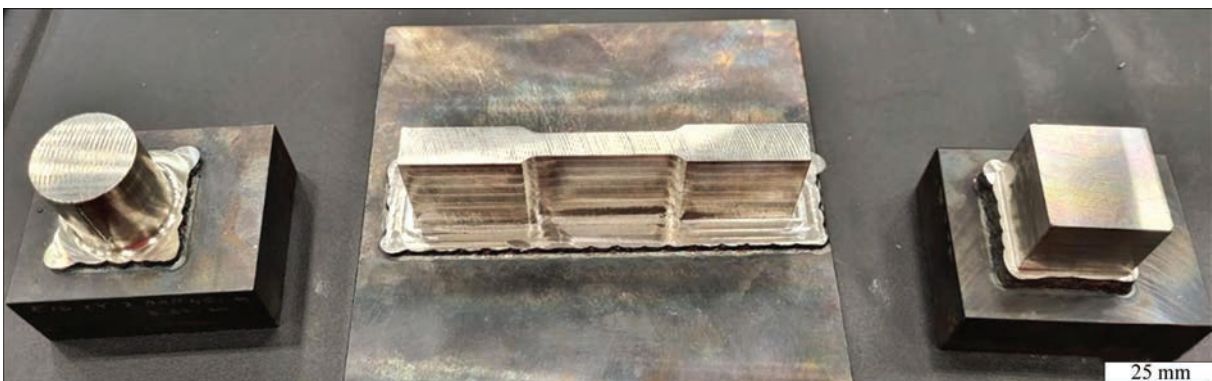
Figure 2. Machined part geometries for: a — hardness; b — tensile, and c — CTE tests
