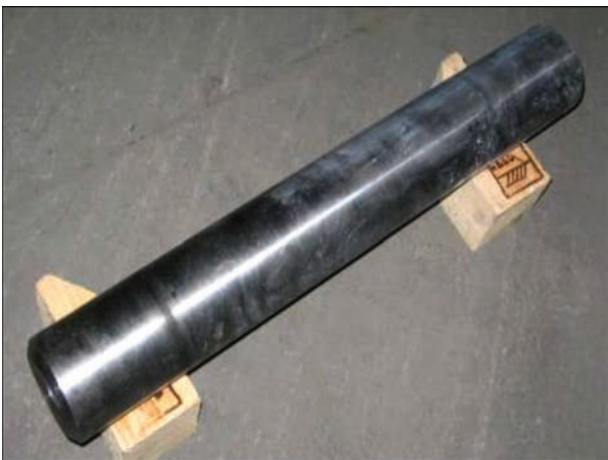
Figure 6. Appearance of machined 110 mm dia ingot of 60Zr-20Ti-20Nb alloy
