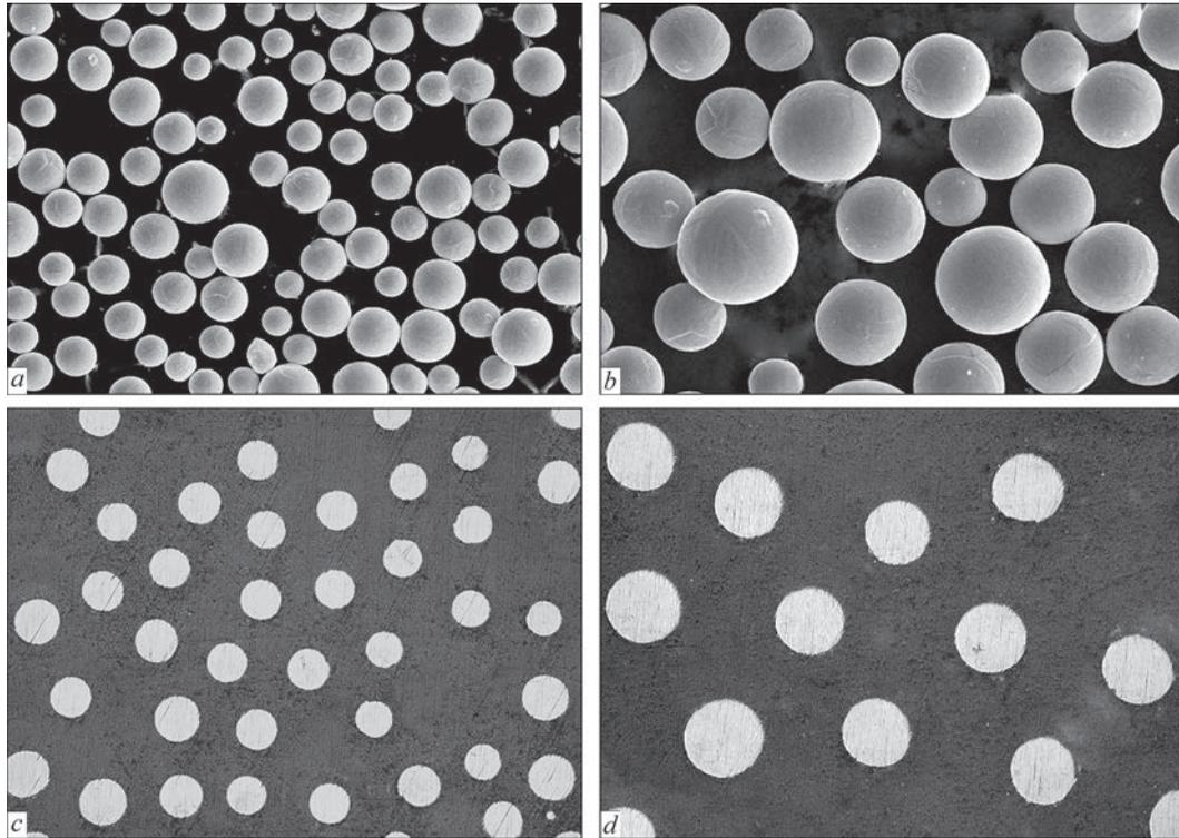
**Figure 3.** SEM images of the morphology (a, b) and microstructure (c, d) of Cp-Ti Grade 2 titanium powder of 106  $\mu\text{m}$  fraction; a, c —  $\times 100$ ; b, d —  $\times 200$
