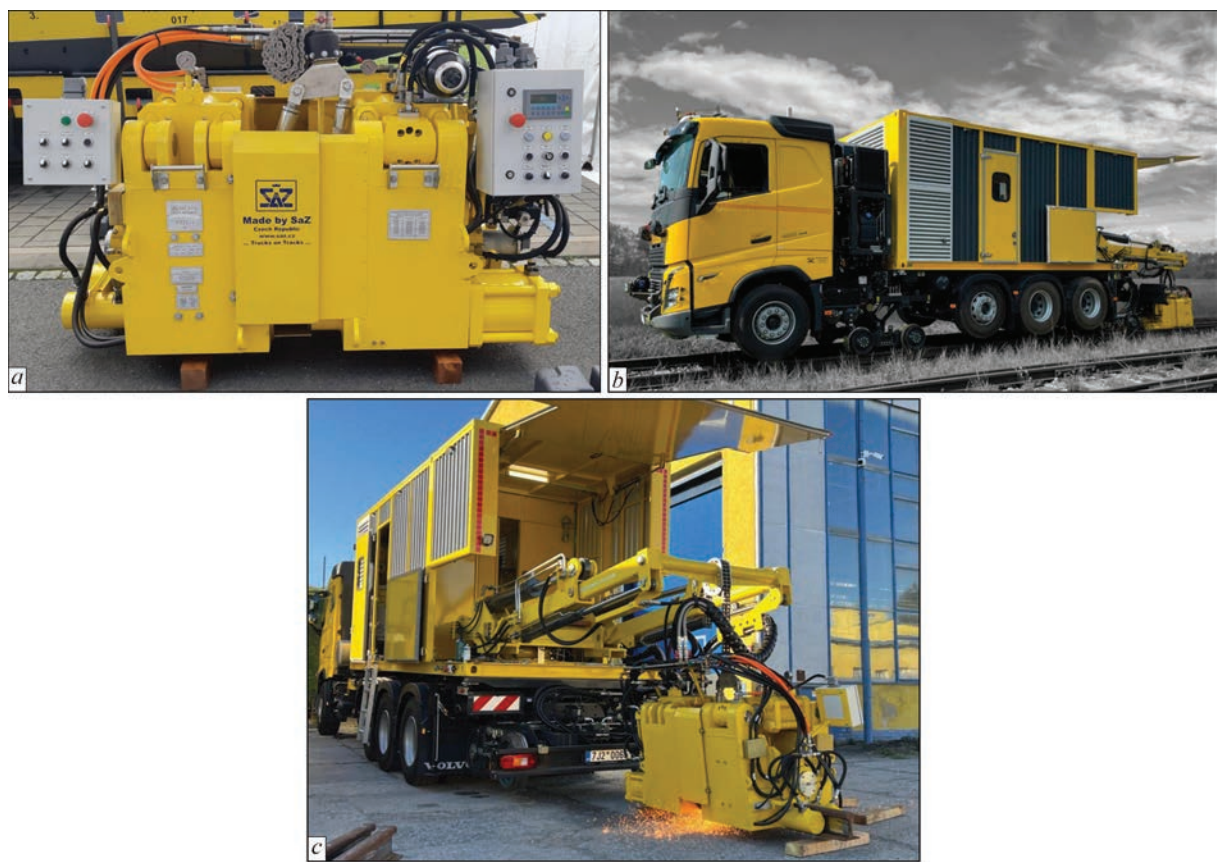
Figure 16. Mobile K922-1 machine (a), double-track WELDERLINER rail welding complex (b, c)
