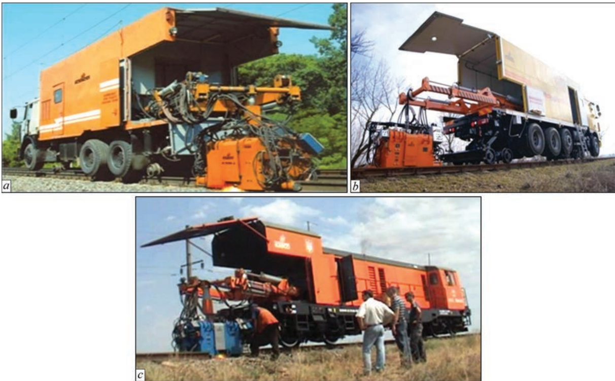
Figure 4. Mobile K922-1 machines as part of rail welding KZM 005 (a), KZM 007 (b) and KRZ 1 (c) complexes
