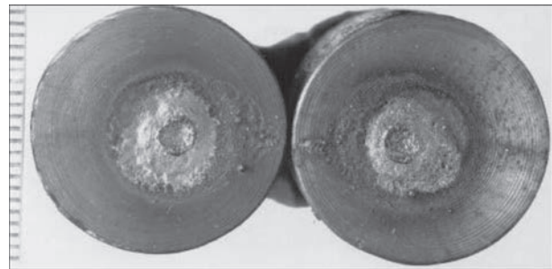
Figure 5. Displacement of the arc to the inner area of the butts
