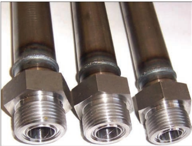
Figure 16. Welding pipes with fittings
