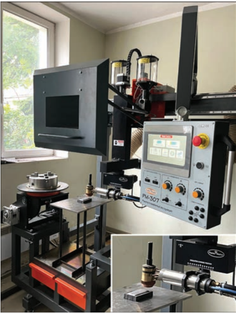
Figure 1. Plasma transferred-arc surfacing unit with two powder feeders and RR-6-03 plasma torch
