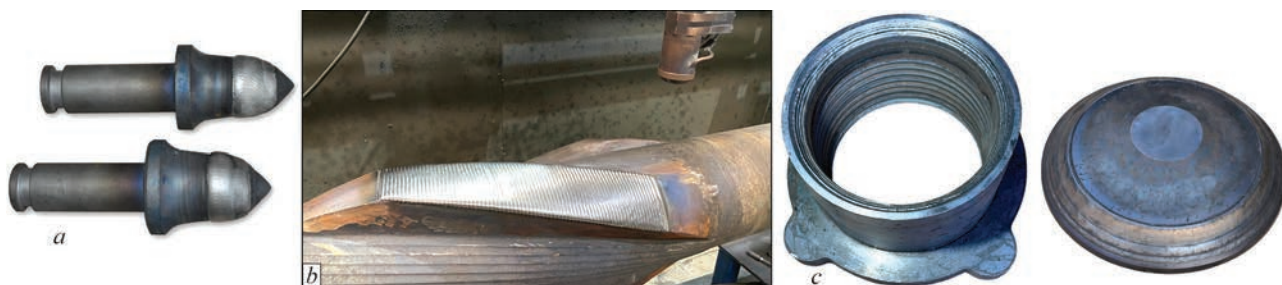
Figure 12. Examples of effective application of PTA surfacing of a composite alloy with 270N15D7Kh3S2 binder alloy: a — tangential cutter; b — calibrator; c — leveling valve of blast furnace
