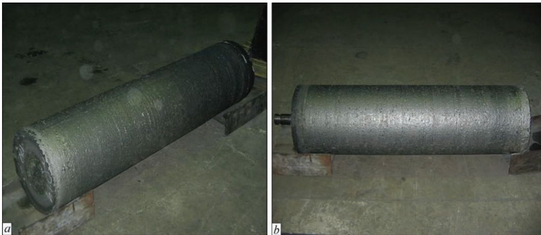
Figure 7. Finished ingots of 400 mm diameter from heat-resistant alloys: a — KhN60VT; b — KhN38VT
