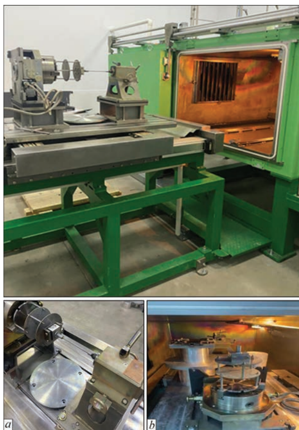
Figure 1. KL-211 installation. Device for assembling and welding gas valve simulator in two spatial positions: with horizontal (a) and vertical axis of rotation (b)
