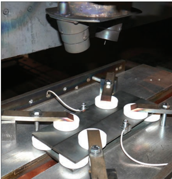
Figure 5. Experimental measurement of the beam power shielded by the process pad
