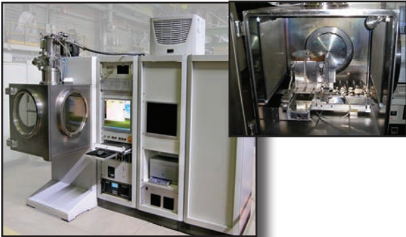
CB 112 mashine: 0.3 m³, 60 kV, up to 15 kW
