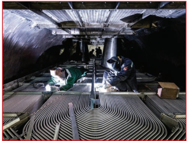
Welding technologies of the PWI in the manufacture of equipment for nuclear power plants
